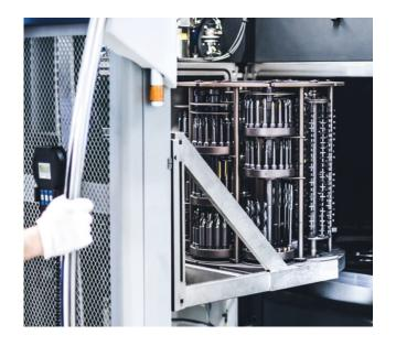
Only an optimum coating of the tool surfaces ensures high-quality cutting surfaces with calculable wear, a long lifetime of the cut and a long service life of your tool.
